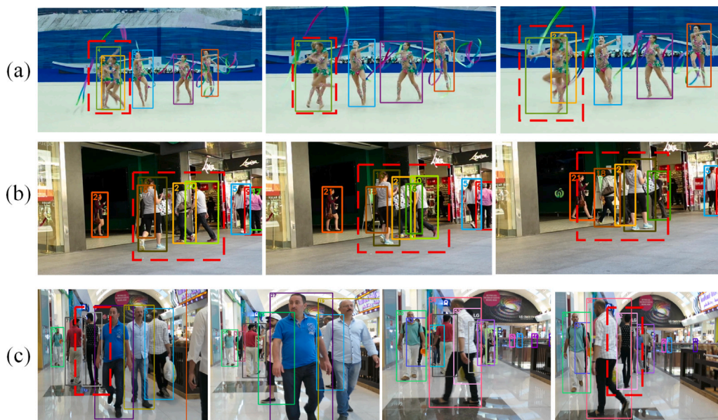
Fig. 1. Challenges and Difficulties in MOT. (a) The red dashed line shows that after Object 2 obscures Object 4, due to their similar appearances, an ID switch occurs when Object 4 reappears. (b) In the red dashed line, an association error between Object 2 and Object 18 is shown under crowded conditions and frequent occlusion. (c) The red dashed line indicates that after a long period of being obscured, Object 8 reappears and its trajectory is initialized as a new trajectory.
