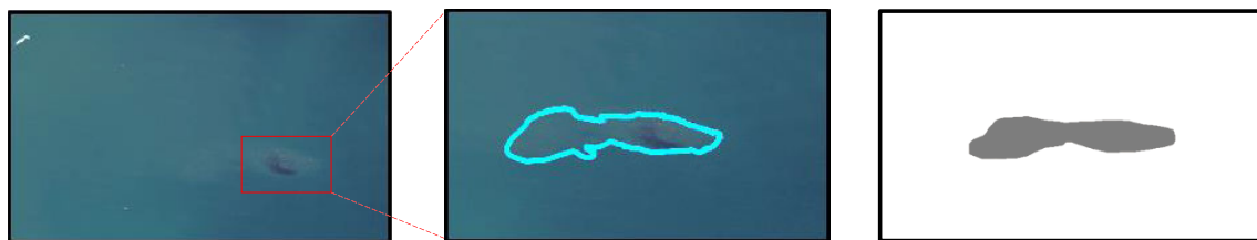
Fig. 9. Symphony oil spill remote sensing data captured by the GF-1 satellite on May 5, 2021, at 10:28 UTC: image, patch, and oil spill position.
