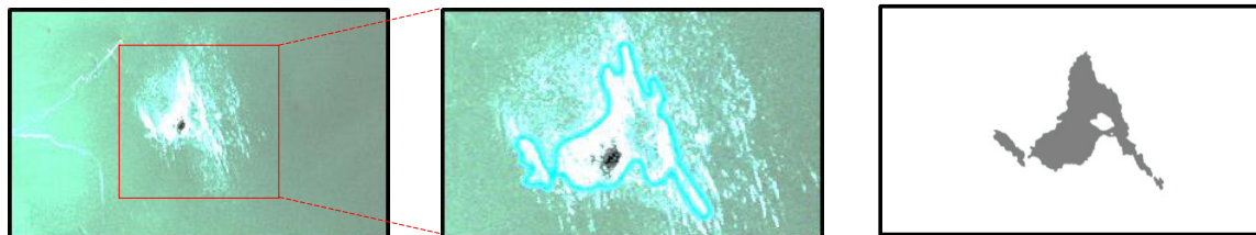
Fig. 8. Symphony oil spill remote sensing data captured by the GF-1 satellite on May 2, 2021 at 10:55 UTC: image, patch, and oil spill position.
