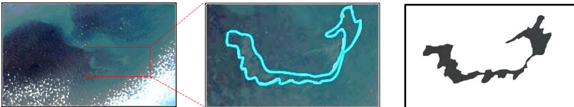
Fig. 12. Sanchi oil spill remote sensing data captured by the GF-1 satellite on January 20, 2018, at 11:17 UTC: image, patch, and oil spill position.
